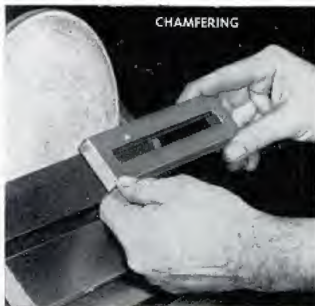
Chamfering corners is done by tilting the sanding table down to 45 deg. Use medium to coarse abrasive
